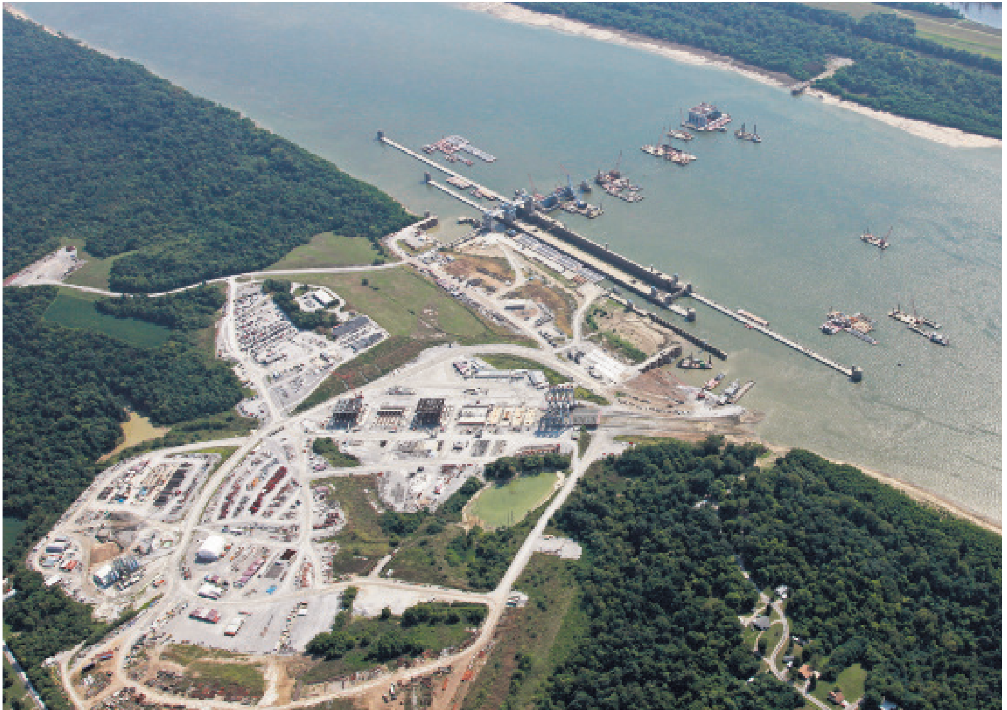
The Olmsted Locks and Dam project's precast yard in Olmsted, Ill., is where the massive shells or pieces of the dam are constructed, and then moved to the shoreline by the super gantry crane and into the Ohio River. There, they are floated by catamaran barge to the dam. The project will replace two of the original locks and is scheduled to open in 2018.
