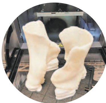
Two hand orthoses printed on a 3D printer at the Albuquerque VA.
