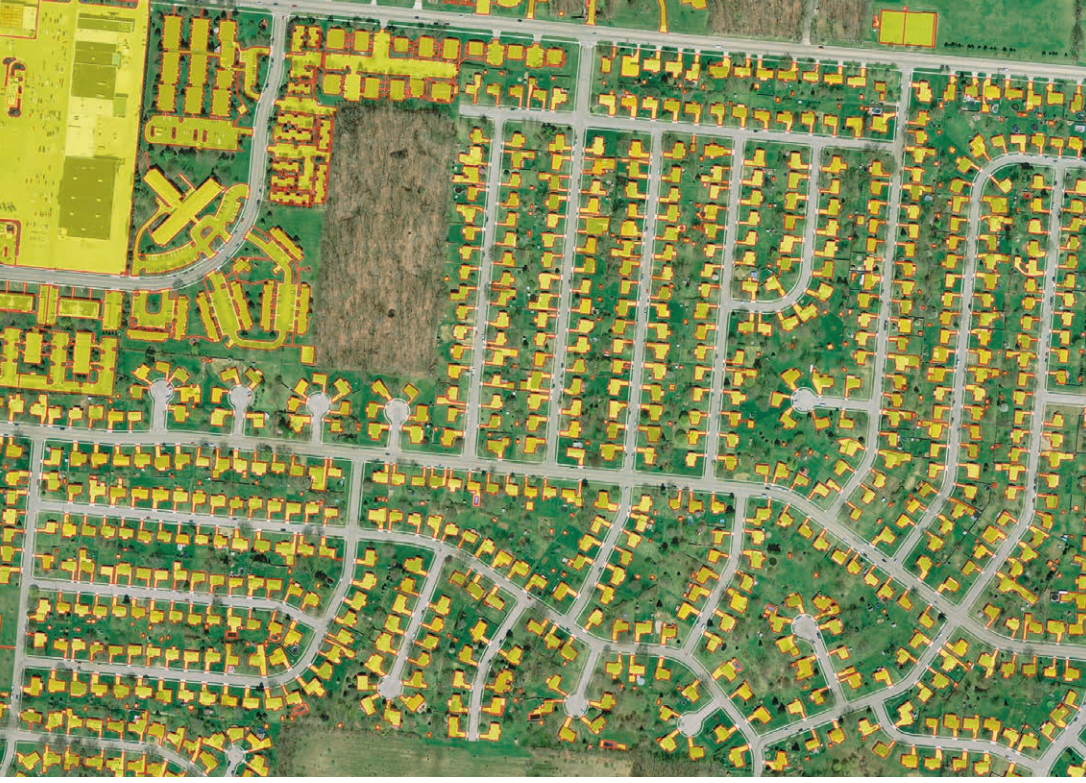
LIDAR impervious surface map of Springfield, Ohio.
