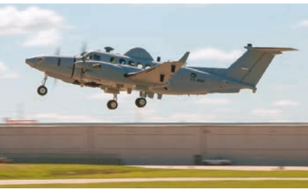
THE BOEING EMARSS airborne ISR platform is among new aircraft being designed to facilitate multi-INT fusion, and is therefore poised to exploit and integrate the next generation of aerial sensors.
